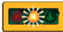
YELLOW: Move into one with a green arrow. If flashin yellow over all lanes: Slow down and proceed with caution.
